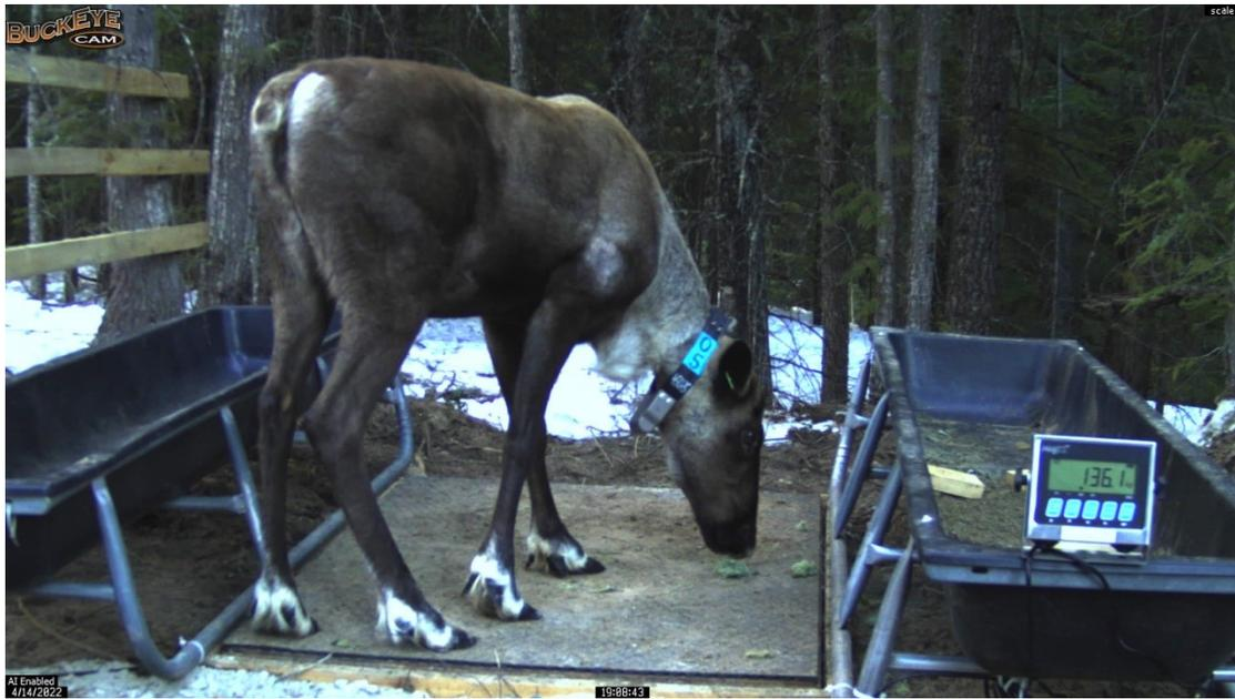
Figure 2: Picture of Cow 05 fully standing on the platform scale, showing her weight on the scale reader.
